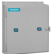
Duplex starter w/o alternator, Size 4, Three phase full voltage, Solid-state overload relay, OLR amp range 50-200A, 240V 50Hz / 277V 60Hz coil, Non-combination type, Enclosure NEMA type 1, Indoor general purpose use
