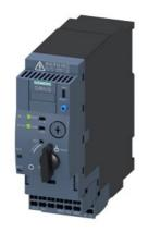
SIRIUS Compact load feeder DOL starter 690 V 110...240 V AC/DC 50...60 Hz 8...32 A IP20 Connection main circuit: plug-in, without terminals Connection auxiliary circuit: Spring-type terminal
