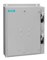
Duplex starter w/o alternator Size 1 Three phase full voltage Solid-state overload relay OLR amp range 3-12A 240VAC 50Hz / 277VAC 60Hz Coil Combination type Two 30A disconnect switches Encl NEMA type 4X 304 S. Steel Water/dust tight non-corrosive
