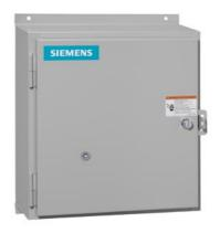
Reversing motor starter, Size 2, Three phase full voltage, Solid-state overload relay, OLR amp range 13-52A, 24VAC 50-60Hz coil, Non-combination type, Enclosure type 4X fiberglass, Water/dust tight noncorrosive, Standard width enclosure
