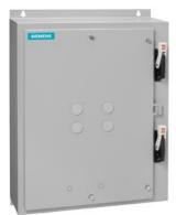
Duplex starter w/o alternator, Size 2 1/2, Three phase full voltage, Solid-state overload relay, OLR amp range 25-100A, 380-440/440-480V 50/60Hz coil, Combination type, Two 100A circuit breakers, Enc NEMA type 4 painted steel, Water/dust tight for outdoors
