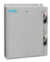
Duplex starter w/o alternator, Size 0, Three phase full voltage, Solid-state overload relay, OLR amp range 3-12A, 110V 50Hz / 120V 60Hz coil, Combination type, Two 10A circuit breakers, Encl NEMA type 4X 304 S-Steel, Water/dust tight noncorrosive
