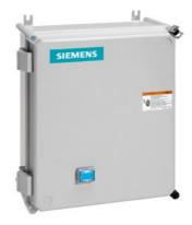
Non-reversing motor starter, Size 0, Three phase full voltage, Solid-state overload relay, OLR amp range 0.25-1A, Non-combination type, Enclosure type 4X fiberglass, Water/dust tight noncorrosive, Standard width enclosure
