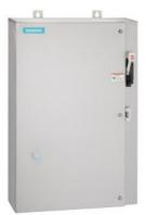
Reversing motor starter, Size 3, Three phase full voltage, Solid-state overload relay, OLR amp range 25-100A, 110V 50Hz / 120V 60Hz coil, Combination type, 125A circuit breaker, Encl NEMA type 4X 304 S-Steel, Water/dust tight noncorrosive
