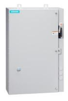
Non-reversing motor starter, Size 3, Three phase full voltage, Solid-state overload relay, OLR amp range 25-100A, 208VAC 60Hz coil, Combination type, 125A circuit breaker, Encl NEMA type 4X 304 S-Steel, Water/dust tight noncorrosive, Standard width enclosure
