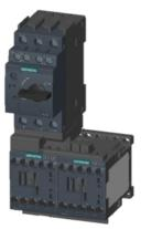
Fuseless motor starter Reversing operation 600VAC Size S00 0.9-1.25A 24V DC screw connection For screw mounting Or 35 mm rail-mounting Type of coordination 2 IQ = 150 KA Also full fills type Of coordination 1 1NO+1NC (MSP) 1NC (per contactor)
