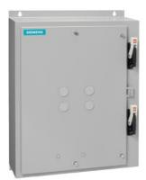
Duplex starter w/o alternator, Size 0, Three phase full voltage, Solid-state overload relay, OLR amp range 5.5-22A, 110V 50Hz / 120V 60Hz coil, Combination type, Two 25A circuit breakers, Enc NEMA type 4 painted steel, Water/dust tight for outdoors
