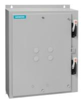
Duplex starter w/o alternator Size 3.5 Three phase full voltage Solid-state overload relay OLR amp range 50-200A 240VAC 50Hz / 277VAC 60Hz Coil Combination type Two 200A disconnect switches Enclosure NEMA type 1 Indoor general purpose use
