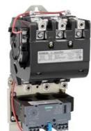
Non-reversing motor starter Size 2 1/2 Three phase full voltage Solid-state overload relay OLRelay amp range 25-100A 190-220/220-240V 50/60HZ coil Combination type No enclosure
