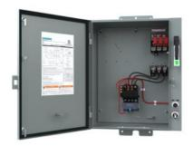
Pump control panel, Size 1 3/4, Three phase full voltage, Solid-state overload relay, OLR amp range 10-40A, 380-440/440-480V 50/60Hz coil, Standard type contactor, 30A fusible disconnect, 30A/600V fuse clip, HOA Sel Sw. <(>&<)> Start P.B., Enclosure NEMA type 3/3R, Weather proof outdoor use
