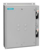
Duplex starter w/ alternator, Size 1 3/4, Three phase full voltage, Solid-state overload relay, OLR amp range 10-40A, 110V 50Hz / 120V 60Hz coil, Combination type, Two 40A circuit breakers, Encl NEMA type 4X 304 S-Steel, Water/dust tight noncorrosive
