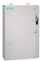
Non-reversing motor starter, Size 2 1/2, Three phase full voltage, Solid-state overload relay, OLR amp range 25-100A, 24VAC 50-60Hz coil, Combination type, 100A non-fusible disconnect, Encl NEMA type 4X 304 S-Steel, Water/dust tight noncorrosive, Extra-wide enclosure
