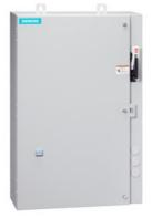
Non-reversing motor starter, Size 2 1/2, Three phase full voltage, Solid-state overload relay, OLR amp range 25-100A, 110V 50Hz / 120V 60Hz coil, Combination type, 100A fusible disconnect, 100A/600V fuse clip, Enclosure NEMA type 4/12, Water/dust tight for outdoors, Extra-wide enclosure
