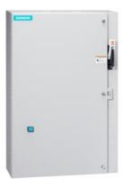
Non-reversing motor starter, Size 3, Three phase full voltage, Solid-state overload relay, OLR amp range 25-100A, Combination type, 100A fusible disconnect, 100A/250V fuse clip, Enclosure NEMA type 1, Indoor general purpose use, Extrawide enclosure
