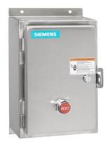
Reversing motor starter, Size 2 1/2, Three phase full voltage, Amb. compensate bimetal OLR, Contactor amp rating 60A, 110V 50Hz / 120V 60Hz coil, Noncombination type, Encl. type 4X 304 S. Steel, Water/dust tight noncorrosive
