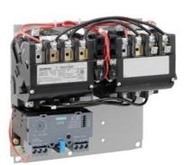
Reversing motor starter Size 1 Three phase full voltage Solid-state overload relay OLRelay amp range 0.75-3.4A 240VAC 50HZ / 277VAC 60HZ coil Non-combination type Enclosure type (open)
