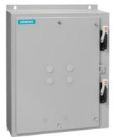
Duplex starter w/o alternator Size 0 Three phase full voltage Solid-state overload relay OLR amp range 0.75-3.4A 240VAC 50Hz / 277VAC 60Hz Coil Combination type Two 30A disconnect switches Encl NEMA type 4X 304 S. Steel Water/dust tight non-corrosive
