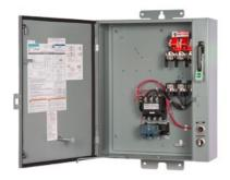
Pump control panel, Size 2, Three phase full voltage, Solid-state overload relay, OLR amp range 13-52A, 110-120/220-240VAC 60Hz coil, Standard type contactor, 60A fusible disconnect, 60A/250V fuse clip, HOA Sel Sw. <(>&<)> Start P.B., Enclosure NEMA type 3/3R, Weather proof outdoor use
