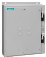
Duplex starter w/o alternator Size 1 Three phase full voltage Solid-state overload relay OLR amp range 5.5-22A 208VAC 60Hz Coil Combination type Two 30A disconnect switches Enclosure NEMA type 4/12 Water/dust tight weather proof
