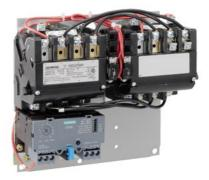
Reversing motor starter Size 1 Three phase full voltage Solid-state overload relay OLRelay amp range 10-40a 220-240/440-480VAC 60HZ coil Non-combination type Enclosure type (open)
