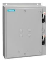
Duplex starter w/o alternator, Size 0, Three phase full voltage, Solid-state overload relay, OLR amp range 3-12A, 24VAC 50-60Hz coil, Combination type, Two 10A circuit breakers, Encl NEMA type 4X 304 S-Steel, Water/dust tight noncorrosive
