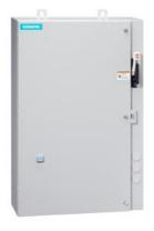
Non-reversing motor starter, Size 1, Three phase full voltage, Solid-state overload relay, OLR amp range 3-12A, 24VAC 50-60Hz coil, Combination type, 30A fusible disconnect, 30A/600V fuse clip, Encl NEMA type 4X 304 S-Steel, Water/dust tight noncorrosive, Extra-wide enclosure
