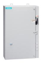
Non-reversing motor starter, Size 2 1/2, Three phase full voltage, Solid-state overload relay, OLR amp range 25-100A, Combination type, 100A circuit breaker, Enclosure NEMA type 4/12, Water/dust tight for outdoors, Standard width enclosure
