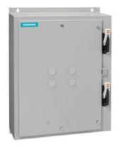
Duplex starter w/o alternator Size 4 Three phase full voltage Solid-state overload relay OLR amp range 50-200A 240VAC 50Hz / 277VAC 60Hz Coil Combination type Two 200A disconnect switches Encl NEMA type 4 painted steel Water/dust tight weather proof
