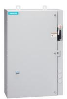
Non-reversing motor starter Size 1 Three phase full voltage Solid-state overload relay OLRelay amp range 3-12A 110-120/220-240VAC 60HZ coil Combination type 10Amp circuit breaker Encl NEMA type 4X 316 S-steel Water/dust tight noncorrosive Extra-wide enclosure
