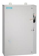
Non-reversing motor starter, Size 4, Three phase full voltage, Solid-state overload relay, OLR amp range 50-200A, 240V 50Hz / 277V 60Hz coil, Combination type, 150A circuit breaker, Encl NEMA type 4X 304 S-Steel, Water/dust tight noncorrosive, Standard width enclosure
