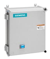
Non-reversing motor starter, Size 1, Three phase full voltage, Solid-state overload relay, OLR amp range 3-12A, 24VDC coil, Non-combination type, Enclosure type 4X fiberglass, Water/dust tight noncorrosive, Standard width enclosure
