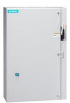
Non-reversing motor starter, Size 2 1/2, Three phase full voltage, Solid-state overload relay, OLR amp range 25-100A, 240V 50Hz / 277V 60Hz coil, Combination type, 100A fusible disconnect, 100A/600V fuse clip, Enclosure NEMA type 1, Indoor general purpose use, Extra-wide enclosure
