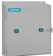
Duplex starter w/o alternator, Size 3, Three phase full voltage, Solid-state overload relay, OLR amp range 25-100A, 190-220/220-240V 50/60Hz coil, Non-combination type, Enclosure NEMA type 1, Indoor general purpose use
