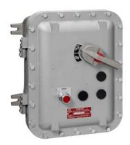
Non-reversing motor starter Size 4 Three phase full voltage Solid-state overload relay OLRelay amp range 50-200A 110VAC 50HZ / 120VAC 60HZ coil Combination type 200A non-fusible disconnect Encl NEMA type 4X Fiberglass Water/dust tight non-corrosive Standard width enclosure
