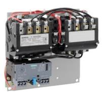
Reversing motor starter Size 1 Three phase full voltage Solid-state overload relay OLRelay amp range 5.5-22A 190-220/220-240V 50/60HZ coil Non-combination type Enclosure type (open)
