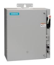
Pump control panel, Size 5, Three phase full voltage, Solid-state overload relay, OLR amp range 55-250A, 220-240V 50-60Hz/DC coil, Standard type contactor, 400A circuit breaker, HOA Sel Sw. <(>&<)> Start P.B., Enclosure NEMA type 3/3R, Weather proof outdoor use
