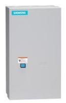
Reversing motor starter, Size 3 1/2, Three phase full voltage, Solid-state overload relay, OLR amp range 50-200A, Non-combination type, Enclosure type 1, Indoor general purpose use, Standard width enclosure
