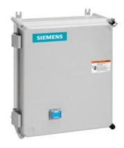
Non-reversing motor starter, Size 1, Three phase full voltage, Solid-state overload relay, OLR amp range 0.75-3.4A, 110V 50Hz / 120V 60Hz coil, Non-combination type, Enclosure type 4X fiberglass, Water/dust tight noncorrosive, Standard width enclosure
