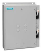
Duplex starter w/o alternator Size 0 Three phase full voltage Solid-state overload relay OLR amp range 3-12A Combination type Two 30A disconnect switches Encl NEMA type 4 painted steel Water/dust tight weather proof
