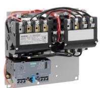
Reversing motor starter Size 1 Three phase full voltage Solid-state overload relay OLRelay amp range 10-40a 550/575-600 50/60HZ coil Non-combination type Enclosure type (open)
