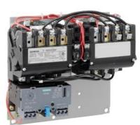
Reversing motor starter Size 0 Three phase full voltage Solid-state overload relay OLRelay amp range 0.25-1A 110-120/220-240VAC 60HZ coil Non-combination type Enclosure type (open)
