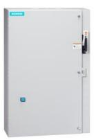
Non-reversing motor starter, Size 2 1/2, Three phase full voltage, Solid-state overload relay, OLR amp range 25-100A, Combination type, 100A circuit breaker, Enclosure NEMA type 1, Indoor general purpose use, Extra-wide enclosure
