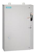
Non-reversing motor starter Size 1 3/4 Three phase full voltage Solid-state overload relay OLRelay amp range 10-40a 208VAC 60HZ coil Combination type 60Amp non-fused disconnect Encl NEMA type 4X 316 S-steel Water/dust tight non-corrosive Extra-wide enclosure
