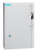
Non-reversing motor starter, Size 2 1/2, Three phase full voltage, Solid-state overload relay, OLR amp range 25-100A, 24VDC coil, Combination type, 100A fusible disconnect, 100A/600V fuse clip, Enclosure NEMA type 1, Indoor general purpose use, Extra-wide enclosure
