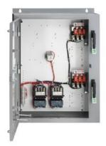
Duplex starter with alternator Size 1 Three phase full voltage Solid-state overload relay OLR amp range 5.5-22A 110VAC 50Hz / 120VAC 60Hz Coil Combination type Two 30A disconnect switches Enclosure NEMA type 1 Indoor general purpose use
