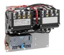
Reversing motor starter Size 0 Three phase full voltage Solid-state overload relay OLRelay amp range 5.5-22A 110-120/220-240VAC 60HZ coil Non-combination type Enclosure type (open)
