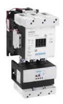
Non-reversing motor starter Size 5 Three phase full voltage Solid-state overload relay OLRelay amp range 55-250A 23-26V 50-60HZ/DC coil Combination type No enclosure
