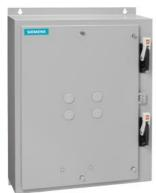
Duplex starter w/o alternator Size 0 Three phase full voltage Solid-state overload relay OLR amp range 0.75-3.4A Combination type Two 30A disconnect switches Enclosure NEMA type 4/12 Water/dust tight weather proof
