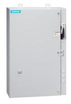
Non-reversing motor starter, Size 4, Three phase full voltage, Solid-state overload relay, OLR amp range 50-200A, Combination type, 200A fusible disconnect, 200A/250V fuse clip, Enclosure NEMA type 4/12, Water/dust tight for outdoors, Standard width enclosure
