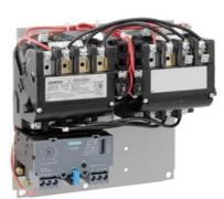
Reversing motor starter Size 0 Three phase full voltage Solid-state overload relay OLRelay amp range 0.25-1A 208VAC 60HZ coil Non-combination type Enclosure type (open)
